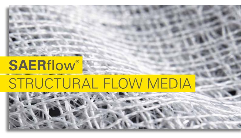
SAERflow combines a glass reinforcement and a lightweight synthetic structure. Together, they provide uncompressible layers with excellent resin flow and high draping properties. SAERflow is used as an internal flow media, which saves a tremendous amount of time. No need to lay-up or release the external flow mesh or its associated consumable layers.
